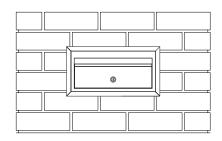
SLEEVE FITS INTO 1.5 BRICK WIDE BY 2 BRICK HIGH CAVITY Build up brickwork to desired height and set letterbox in place
